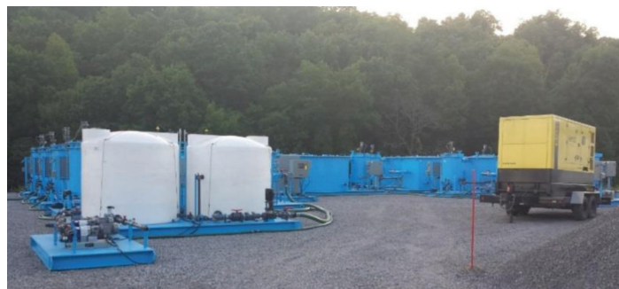
A 100 gpm HydroFlex system is currently being demonstrated in Pennsylvania for production of oil and gas source water from acid mine drainage.
