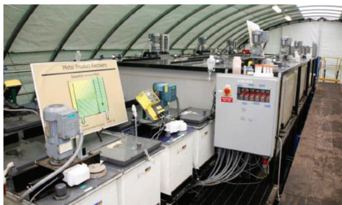
A 30 gpm HydroFlex system was demonstrated in Pennsylvania, processing over one million gallons of mine impacted waters. The sulfate was reduced from ~1,000 mg/L to 133 mg/L. Recovery of the feed water was greater than 98% and process wastes were less than 5% of the incoming feed volume.
